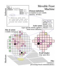
Figure 2: Architectural overview of the movable feast machine used by permission from Ackley (2013a).
